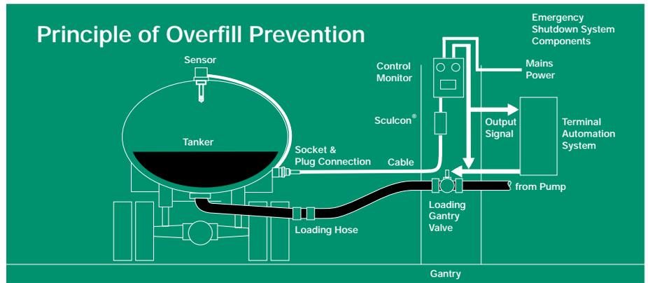
**Scully Five-Wire Optic Sensors** are part of an automatic and continuous self-checking system you can count on. Scully five-wire optic sensors offer all these advantages:
