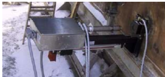
Infrared pyrometers are used to overcome contact measurement
