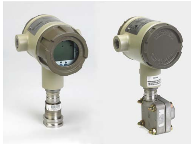
Figure 1 – On the left is an In-line Models STA92L, STA94L and STA97L and on the right is Model STA922, STA940. All Series 900 Absolute Pressure Transmitters feature proven piezoresistive sensor technology
