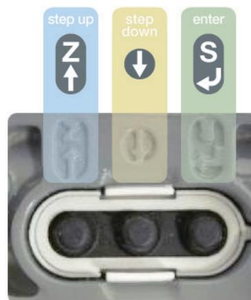
Figure 1: SmartLine Configuration Buttons
