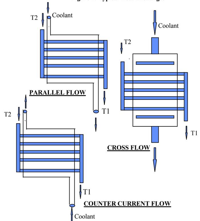
Note: Heat Exchangers shown are for a cooling process. In a heating process the coolant would be replaced by a heating medium and the temperatures T2 and T1 would be reversed.
