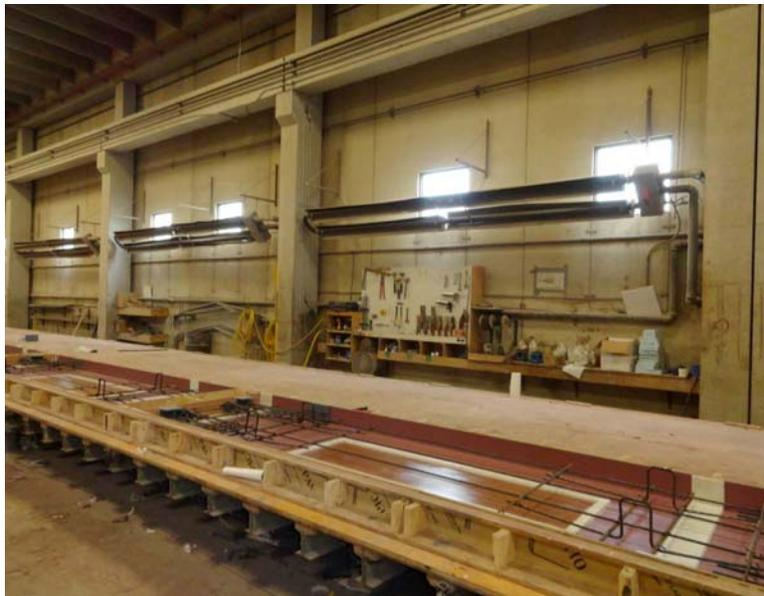
Figure 3. Radiant gas heaters above concrete beds.
