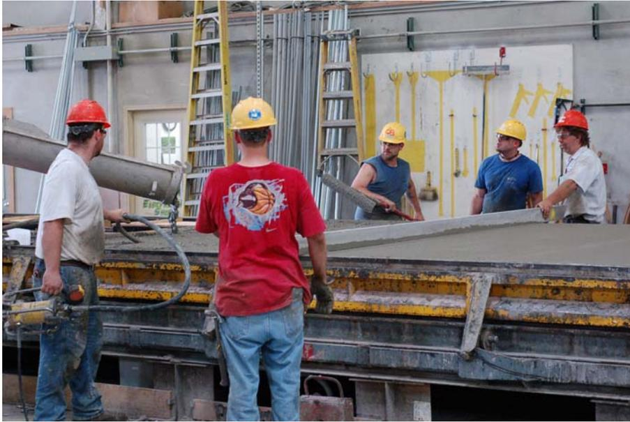
Figure 2. The precast concrete production process involves pouring concrete into molds, or beds, and curing it for a certain period of time.
